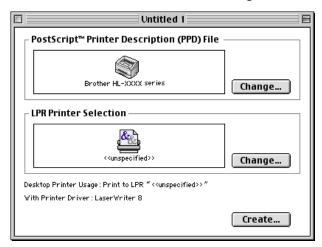
6 Enter the IP address and service name of the printer you are using. When specifying the queue, use the BRN\_XXXXXX\_P1\_AT. XXXXXX are the last six digits of the Ethernet address.
